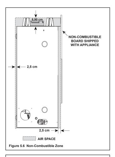
**Note:** AIR SPACE denoted in Figure 5.6 is defined by the nailing tabs and metal standoffs.
